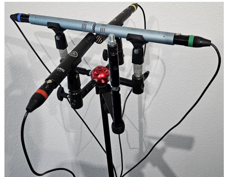
The two pairs of cardioid microphones have been mounted, and the connectors for the four-channel multicore have been connected. You may use separate microphone cables; it doesn't matter. It's more a question of what you have on hand and/or your personal workflow. Make sure the diaphragms of the microphones are as close together as possible. This may vary depending on the microphones used..
